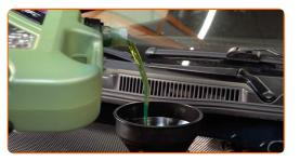
Replacement: engine oil and filter – VW Scirocco II (53B). Tip:
