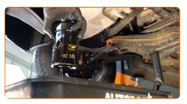
Replacement: engine oil and filter – VW Scirocco II (53B). Tip from AUTODOC experts:
