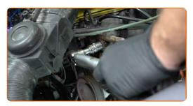
Tighten the water pump pulley fastener. Use HEX No.H6. Use a torque wrench. Tighten it to 9 nm torque.
