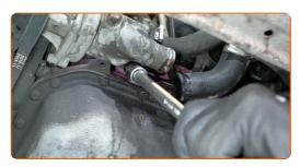
Remove the thermostat housing.
