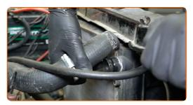
Unscrew the radiator fasteners. Use a drive socket #10. Use a ratchet wrench.
