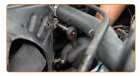
33 Attach the engine cooling fan connector.
