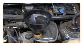
Pour coolant in the coolant reservoir.
