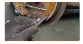
25 Install the hold-down spring. Use round-nose pliers.
