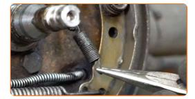
Remove the upper return spring of the brake shoes. Use round-nose pliers.
