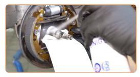
Install the brake drum assembled with the wheel hub bearing.
