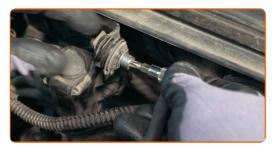
6 Unscrew the brake fluid reservoir cap.
