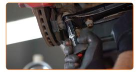
Screw the rear fastener connecting the control arm to the subframe. Use a drive socket #15. Use a drive socket #18. Use a ratchet wrench.
