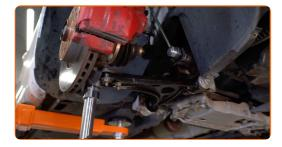
Screw the front arm fastener. Use a drive socket #18. Use a torque wrench. Tighten it to 70 Nm torque.+180°
