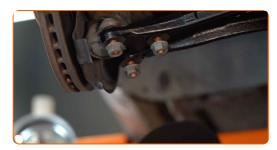
Screw the fasteners of the ball joint. Use a drive socket #15. Use a ratchet wrench.
