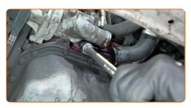
Remove the thermostat housing.
