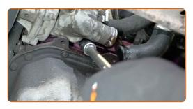
Remove the thermostat housing.
