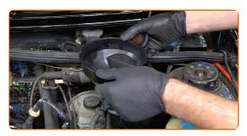
Pour coolant in the coolant reservoir.
