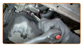
Remove the thermostat housing.
