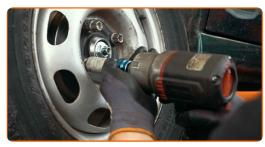
Screw on the hub nut. Use a drive socket #24. Use a ratchet wrench.
