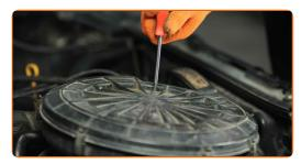
Release the air filter cover clips.
