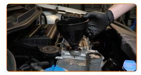
Pour new oil into the engine in the amount recommended by the car manufacturer.
