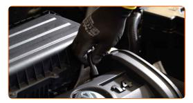
$_{\Lambda}$  Undo the engine cover screws (4 pieces).
