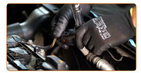
Install the new ignition coil to the spark plug well. Make sure you hear a click indicating that it is locked in place.
