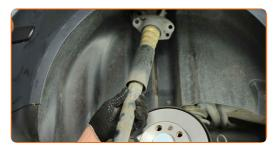
Unscrew the upper fastener of the shock absorber. Use a drive socket #16. Use a ratchet wrench.
