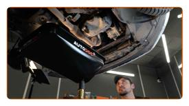
Unscrew the drain plug. Use a drive socket #19. Use a ratchet wrench.
