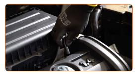
Undo the engine cover screws (4 pieces).
