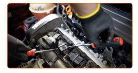
Take out the ignition coil from the spark plug well. Use an ignition coil remover.
