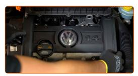
6 Undo the plastic locking tabs of the ignition coil connector.
