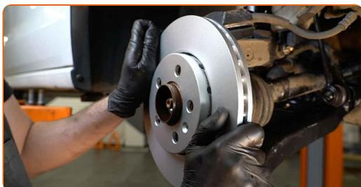
**20** Tighten the brake disc fastening. Use Torx T30. Use a torque wrench. Tighten it to 4 Nm torque.
