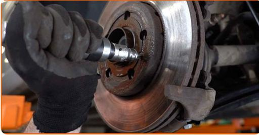
**14** Remove the brake disc.
