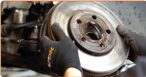
**15** Clean the hub. Use a wire brush. Treat the contacting surface. Use copper grease.
