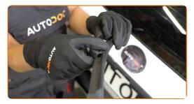
Remove the blade from the wiper arm.
