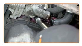
Remove the thermostat housing.
