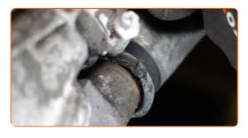
Drain the coolant from the engine.
