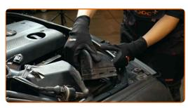
Unscrew the fasteners of the heat shield of the air filter housing. Use a Phillips screwdriver.
