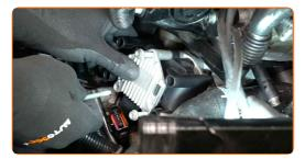
Tighten the ignition coil fastening. Use HEX No.H5. Use a torque wrench. Tighten it to 7 Nm torque.
