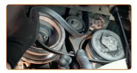
Return the tensioner pulley to its initial position. Use a combination spanner #16.
