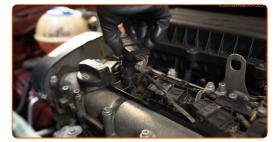
9 Detach the connector from the ignition coil.
