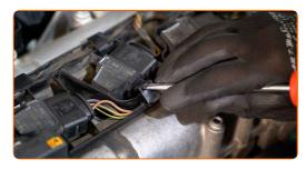
Pry up the ignition coil. Use a flat screwdriver.
