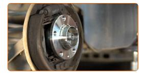
Tighten the hub. Use drive 12-point socket #30. Use a torque wrench. Tighten it to 175 nm torque.
