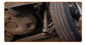
6 Clean the brake drum. Use a wire brush. Use WD-40 spray.
