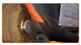
Treat the contacting surface. Use copper grease.
