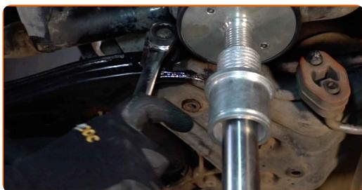
**21** Remove the support from under the engine.
