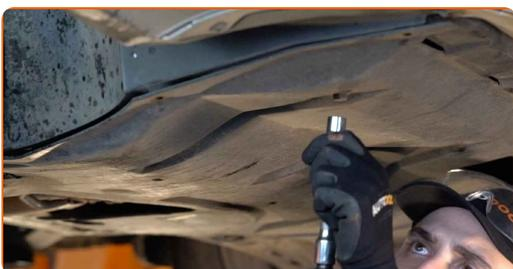
**7** Remove the lower sound insulation.
