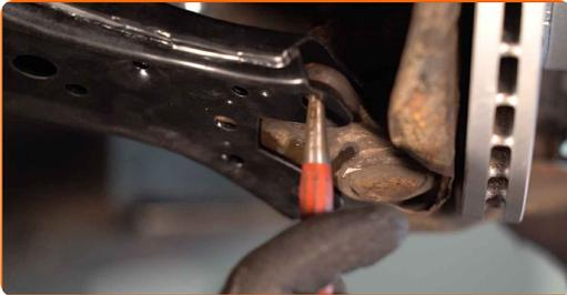
**23** Tighten the fasteners of the ball joint. Use a drive socket #13. Use a torque wrench. Tighten it to 20 Nm torque. +90°
