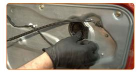
Attach the mirror adjuster connector to the control unit.
