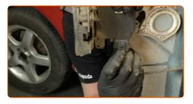
Remove the door lock. Use a flat screwdriver.
