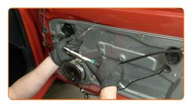
Attach the wiring harness to the protective cover of the door.
