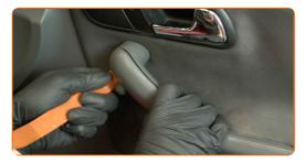
Remove the door armrest screws. Use a Phillips screwdriver.
