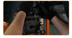
11 Remove the brake caliper.
