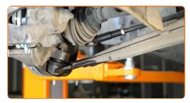
Disconnect the ball joint from the steering knuckle. Use a crowbar. Use a ball joint puller.
