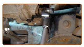
Insert the funnel. Pour the oil into the gearbox through the filler hole. Required amount of oil: 1.5 L.
