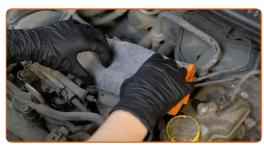
Undo the fastening screws of the air filter cover. Use a Phillips screwdriver.
