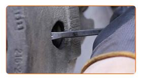
10 Remove the brake caliper.
