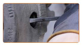
10 Remove the brake caliper.
