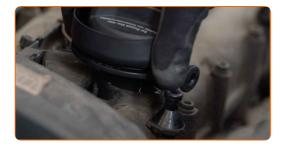
Attach the crankcase ventilation hose to the oil filler neck.
