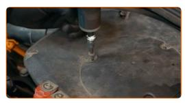
Remove the air filter housing.
