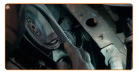
Replacement: serpentine belt – VW Polo III Hatchback (6N2). Tip:
