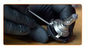
Replacement: headlight bulb – VW Polo III Hatchback (6N2). AUTODOC recommends:
