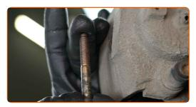
Tighten the brake caliper fasteners. Use HEX No.H6. Use a torque wrench. Tighten it to 25 Nm torque.
