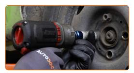
Replacement: brake pads – VW Polo III Hatchback (6N2). Tip from AUTODOC experts:
