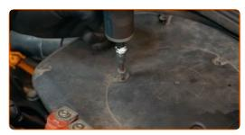
Remove the air filter housing.
