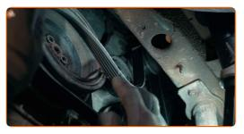
Replacement: serpentine belt – VW Polo III Box Body / Hatchback (6N1). Tip:
