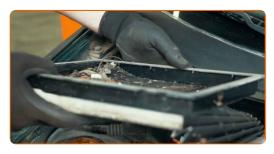
Replacement: pollen filter – VW Polo III Box Body / Hatchback (6N1). Tip from AUTODOC:
