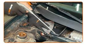
Remove the microfibre cloth from the cabin filter air ducts.
