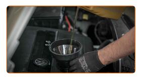
Replacement: engine oil and filter – VW Polo III Box Body / Hatchback (6N1).
