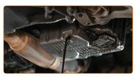
Replacement: engine oil and filter – VW Polo III Box Body / Hatchback (6N1).
