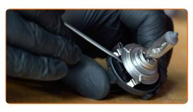
Replacement: headlight bulb – VW Polo III Box Body / Hatchback (6N1).
