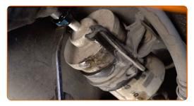
Replacement: fuel filter – VW Polo III Box Body / Hatchback (6N1).
