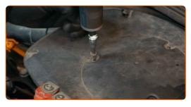
Remove the air filter housing.
