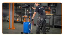
5 Unscrew the drain plug. Use a drive socket No.19 or ring spanner No.19. Drain the used oil.
