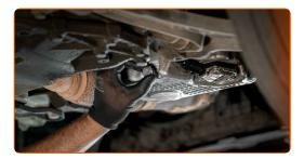
Reinstall the oil pan lower cover. Tighten the fasteners of the oil pan lower cover. Use Torx T25.
