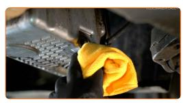
Screw in the new drainage plug and tighten it. Use a drive socket No.19 or ring spanner No.19. Use a torque wrench. Tighten it to 30 nm torque.
