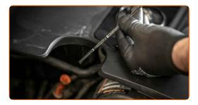
17 Tighten the oil filler cap.
