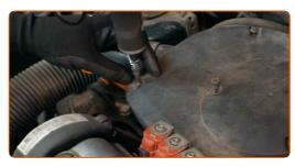
A Remove the air filter housing.
