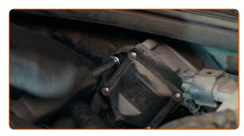
A Remove the ignition coil.
